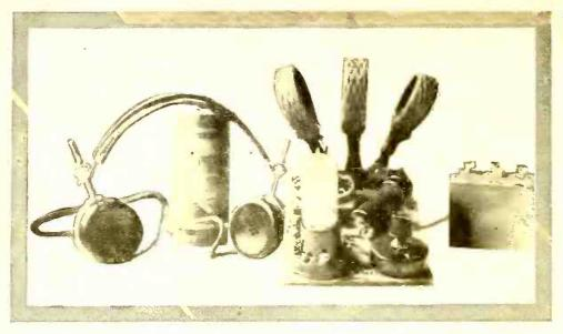
A back view of one of the \$1.00 receivers. Notice the adjustable grid leak and the three honeycomb coils which efficiently received ship-to-shore traffic when the set was plugged into an electric light socket in Chicago.
