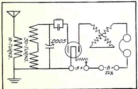
Wiring Diagram for the receiving circuit described by William Vreeland. A four inch tube is used to wind the tuning inductance. Mr. Vreeland has had very good success with this circuit, and for that reason we are passing it along.
