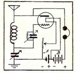
Here is another of the hookups built with the "\$1.00 circuit" by Mr. Perry. This hookup differs fram the one shown on Page 7 in that only one coil is used. This arrangement insures excellent long-distance broadcast reception.
