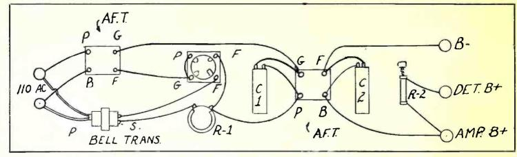
Fig. 2. A one tube "B" voltage rectifier, suitable for sets using no more than three receiving tubes.
