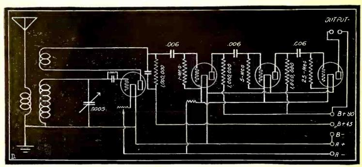
Above is the wiring diagram for the three circuit tuner with three stages of resistance coupled amplification. This method of amplifying gives wonderful, clear tone to the incoming signals.
